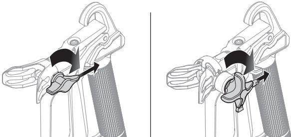
3. Unlock the gun and squeeze the trigger, pointing the gun at a scrap piece of wood or cardboard. This allows pressure in the spray hose to blow out the obstruction. When the nozzle is clear, paint will come out in a straight, high pressure stream.
